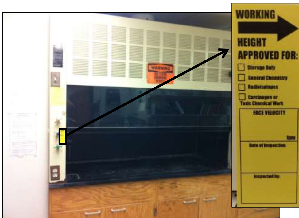
Figure 4.1 – Chemical Fume Hood Sash Approved Working Height
